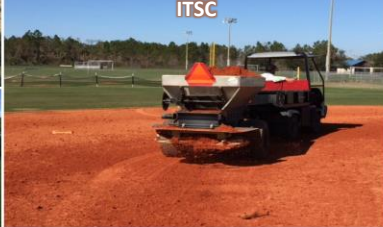
Leveling & grading fresh clay ITSC
