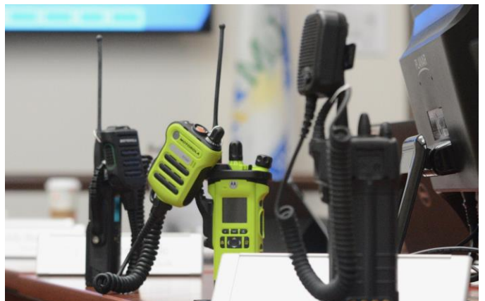
Handheld units for the new radio system. The units, made by Motorola, will have GPS tracking and will be waterproof. The lime ones designed for fire rescue will be intrinsically safe. (Photo by Jonathan Simmons, Palm Coast Observer)
