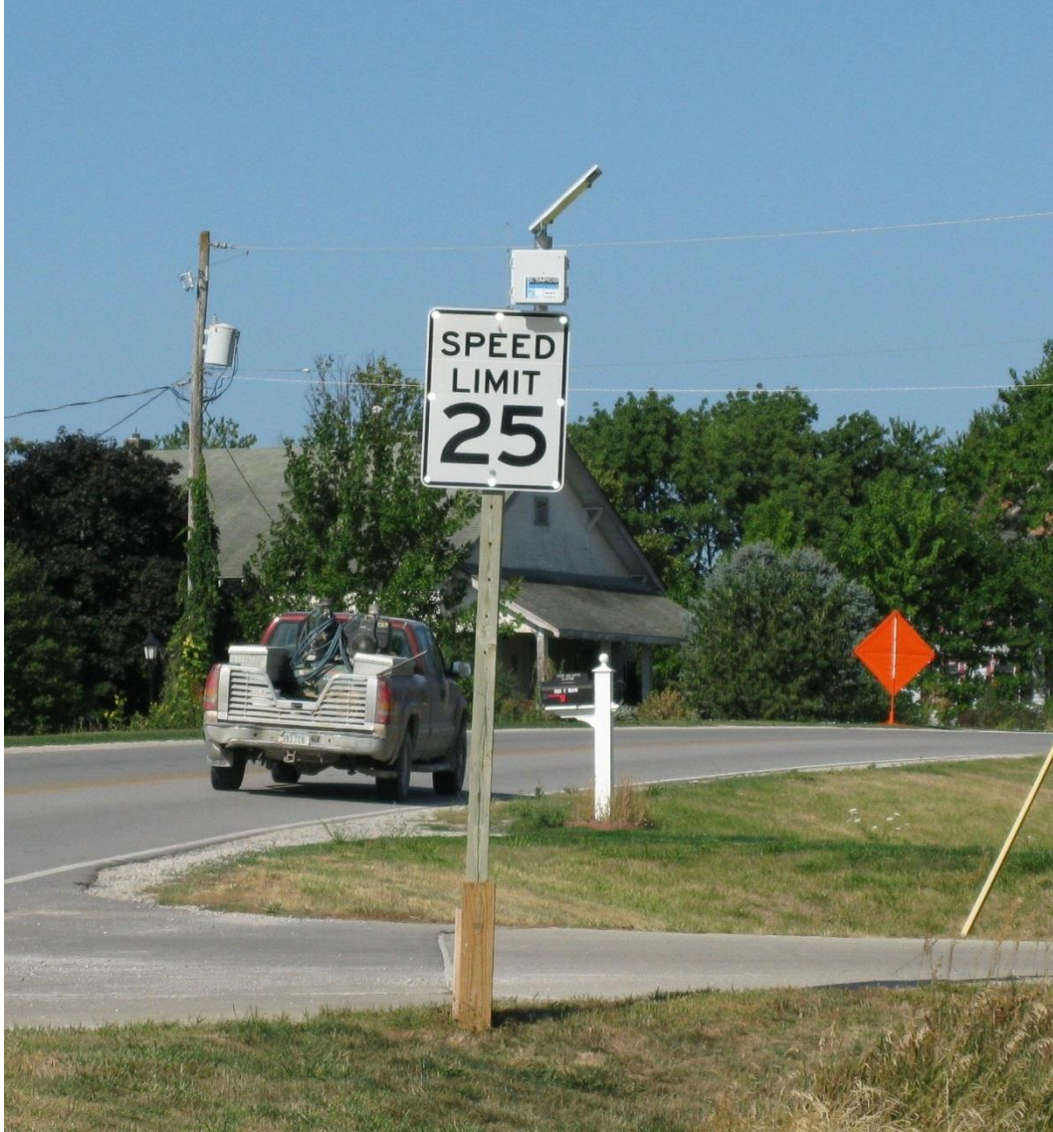
Figure 5-15: Radar-activated LED speed limit sign at east St. Charles community entrance
