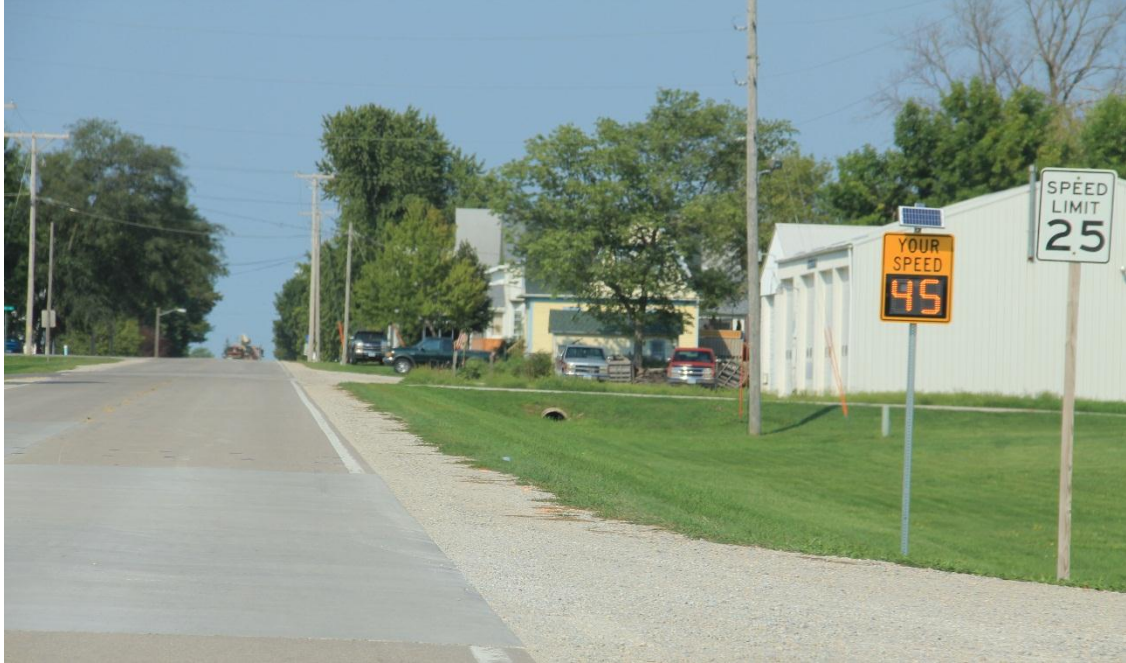
Figure 5-17: DSFS installed at east Rowley community entrance
