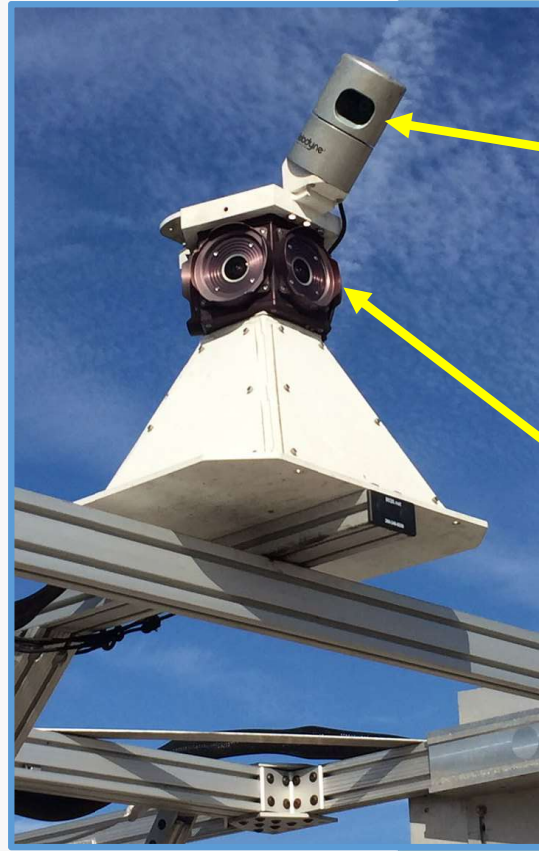
Laser Crack Measurement System (LCMS) •4,000+ point lasers •Length, width, and depth of cracks
