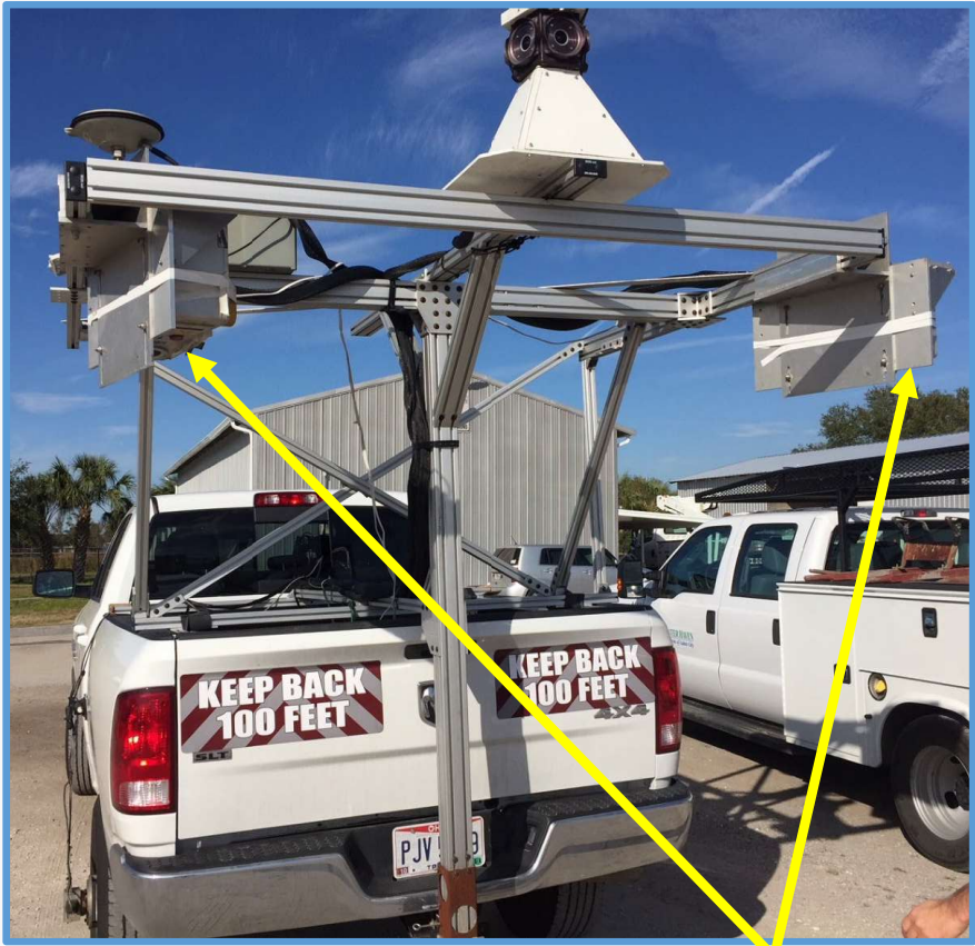
Laser Crack Measurement System (LCMS) •4,000+ point lasers •Length, width, and depth of cracks
