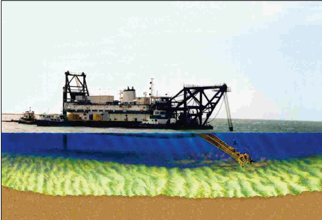
Figure 1. Hydraulic cutterhead pipeline dredge.
