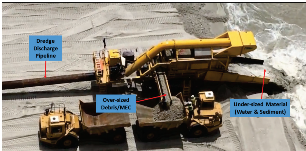
Figure 14. FRS process flow of over and undersized material.
