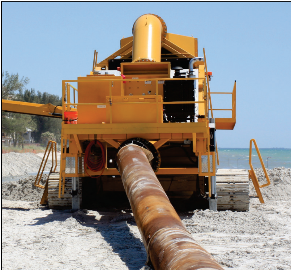
Figure 16. Self-propelled FRS unit mounted on a tracked chassis.
