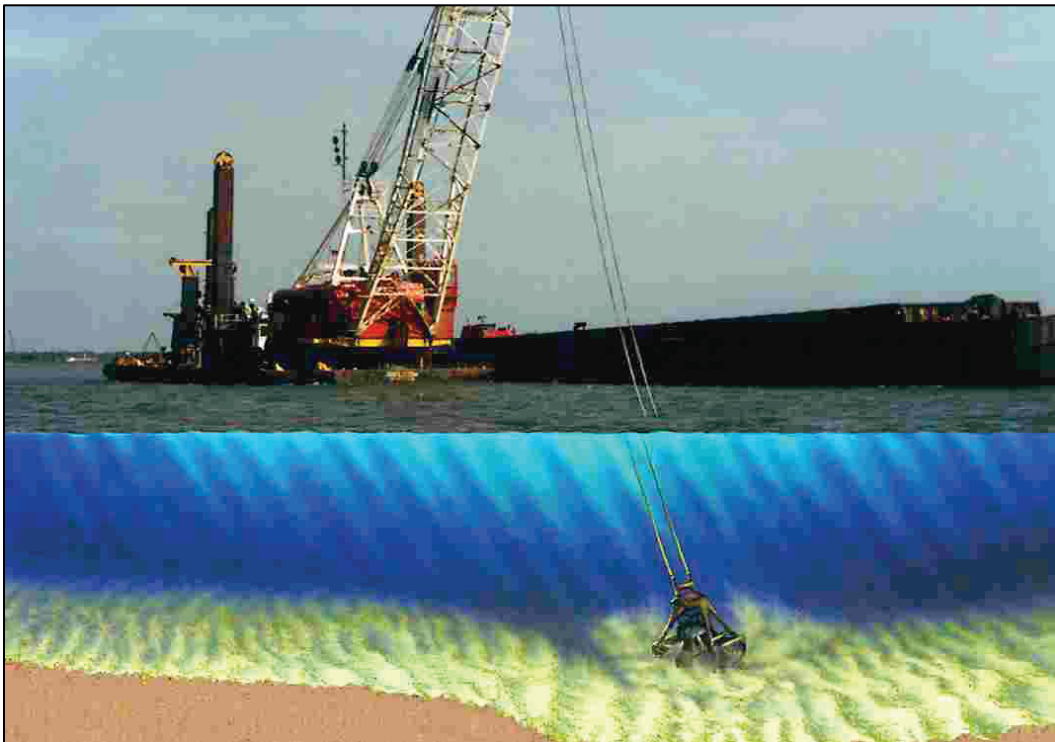
Figure 3. Mechanical (clamshell) dredge.
