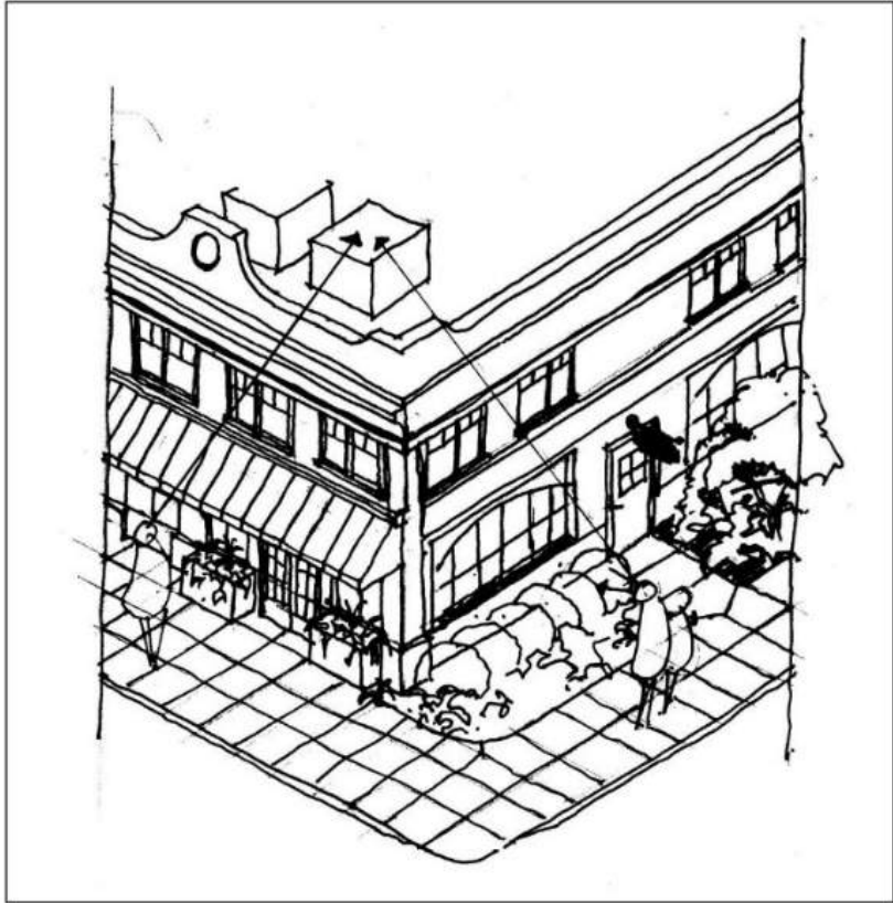
Parapet Screens Rooftop Mechanical
