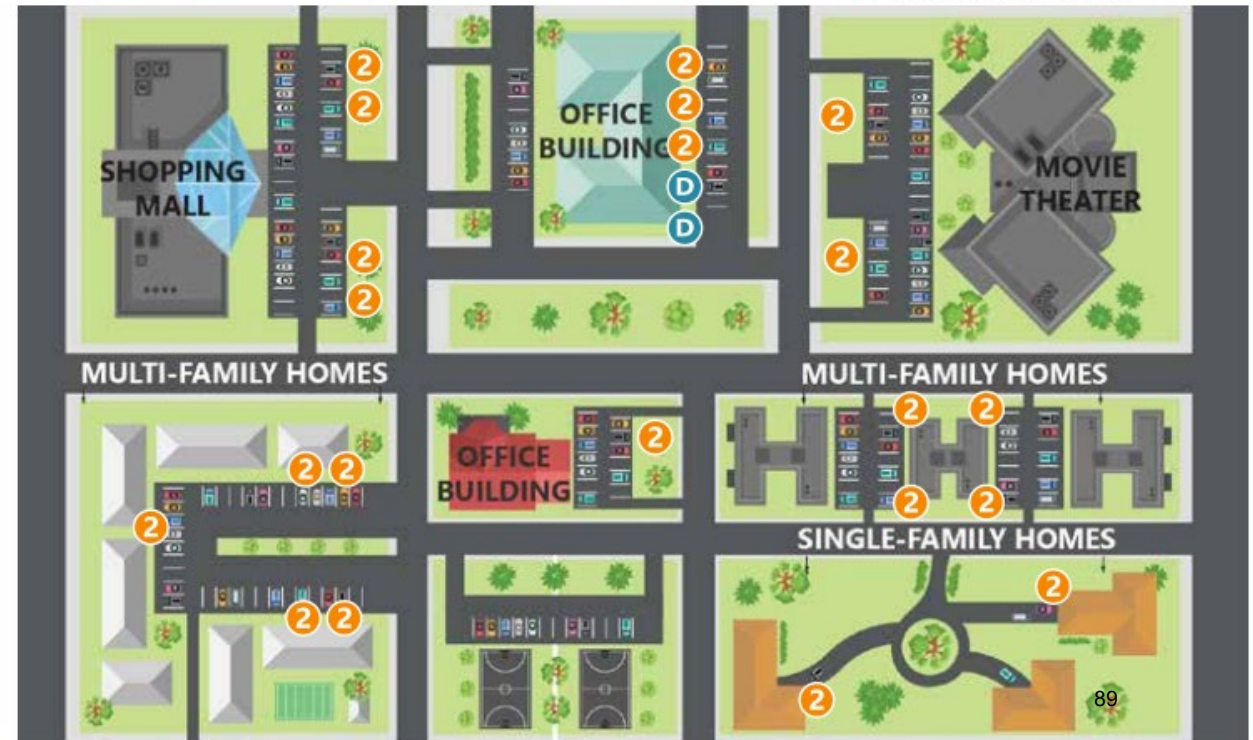
Level 2 Installation Site - Community Charging
