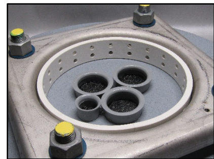
Figure 17-30: Base Plate Design Change Inner Lip Turned Downward
