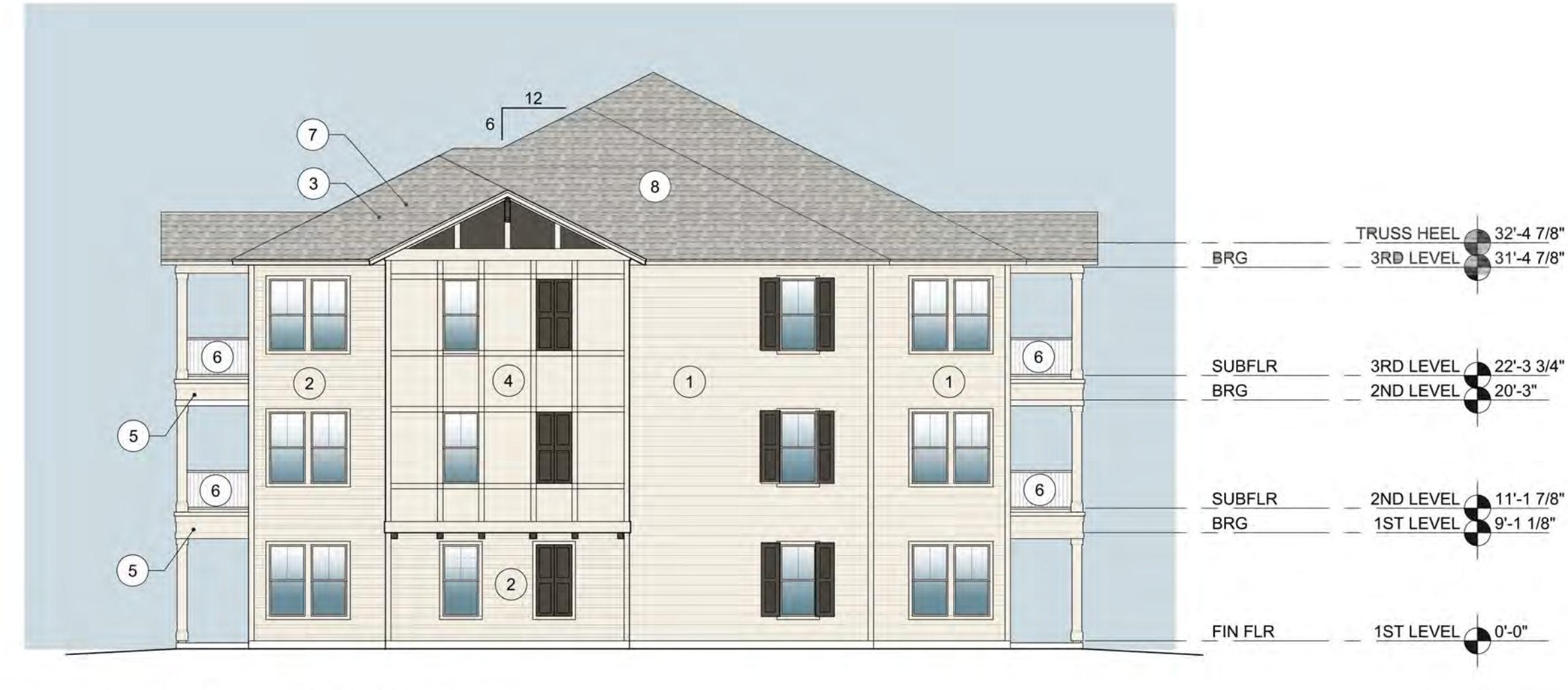
② MIX 1 - EXTERIOR ELEVATION RIGHT
