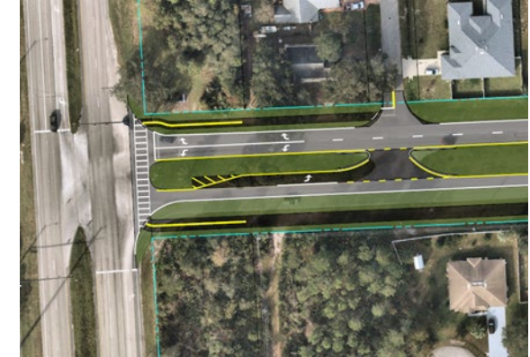
Provide a Path Connection to the Wood Ash Lane to Provide Neighborhood Access
