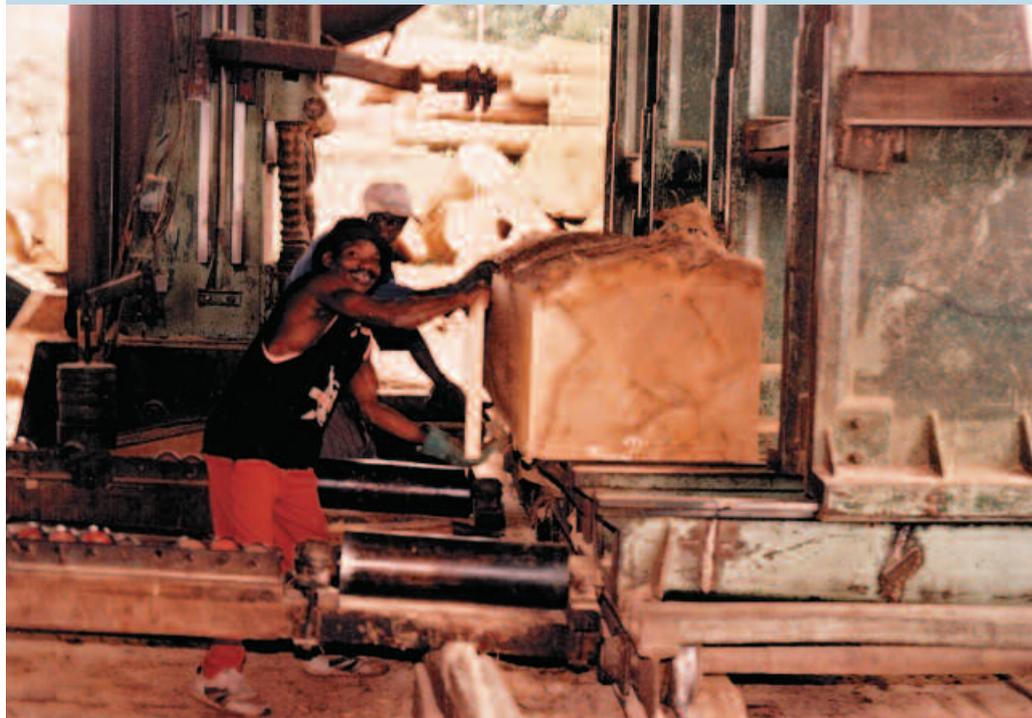
Sawing wawa logs into lumber for the study with a vertical band saw mill.
