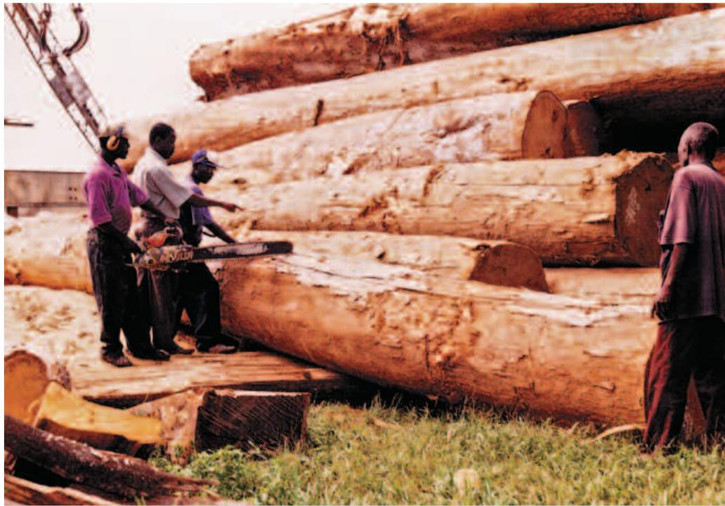
Chain saw operator get specific directives to cross cut logs to the required length.
