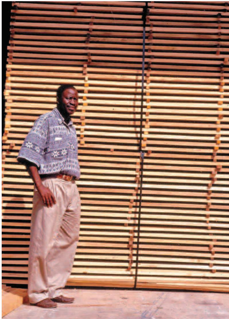
A stack of wawa boards ready for a kiln drying experiment using a 35 m<sup>3</sup> commercial kiln dryer made by Copcal International Dryer Co. (Italy).
