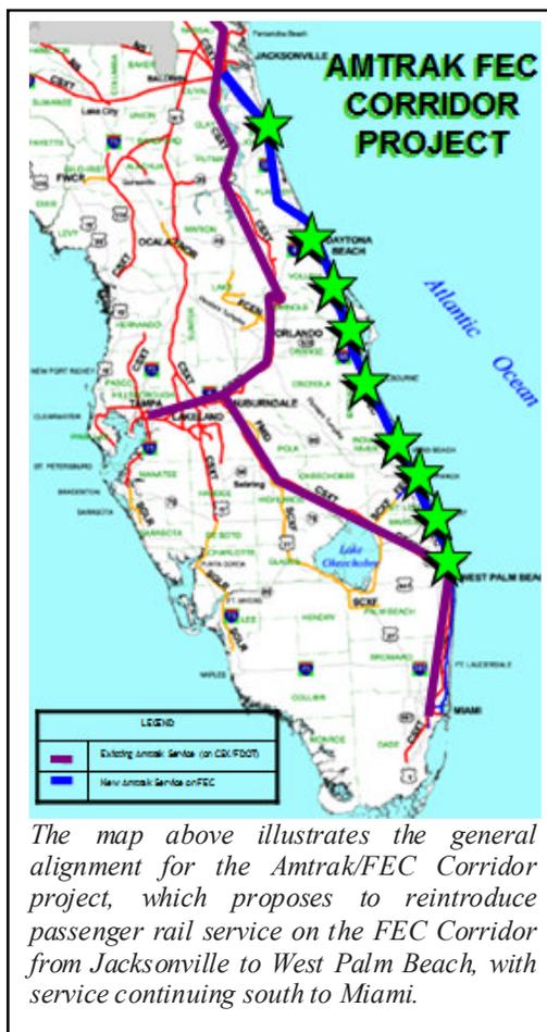
*The map above illustrates the general alignment for the Amtrak/FEC Corridor project, which proposes to reintroduce passenger rail service on the FEC Corridor from Jacksonville to West Palm Beach, with service continuing south to Miami.*
