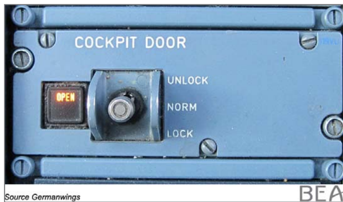
Figure 5 - door control switch
