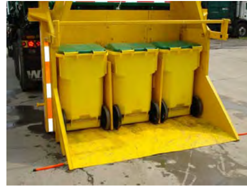
3-65 gallon totes in cart dumper
